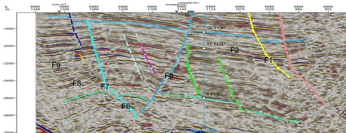
Figure 8. Fault horizon mapping
