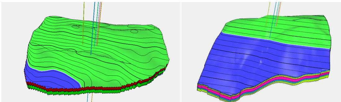
Figure12a: 3D Model of fluid contactfor Reservoir G Figure 12b: 3D Model of fluid contact for Reservoir I
