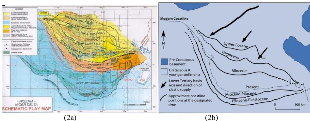
Figure 2(2a) Map of Niger Delta showing the depobelts(2b) Cartoon showing how the coastline of the Niger Delta has prograded since 35Ma. (USGS, The Niger Delta Province).
